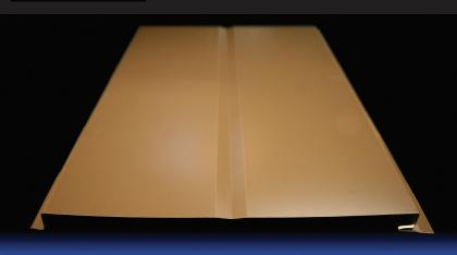
The SWP-12 Soffit-Wall panel is available in smooth and formed surface profiles, flush or reveal at 12" width, 24 gage Grade 50 Galvalume. SWP-12 is a flexible product to meet every architectural design requirement calling for smooth or perforated panels. Architects choose which product will best meet their needs. The flexibility of our Soffit-Wall panel is that it allows for vertical and horizontal open framing or solid substrate installation. Priced to compete, proven to perform.
